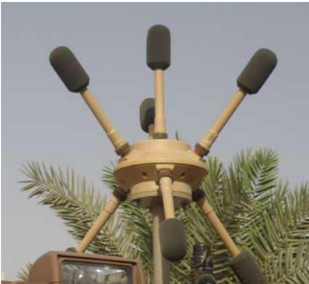
Sniper Detection System sensor mast
