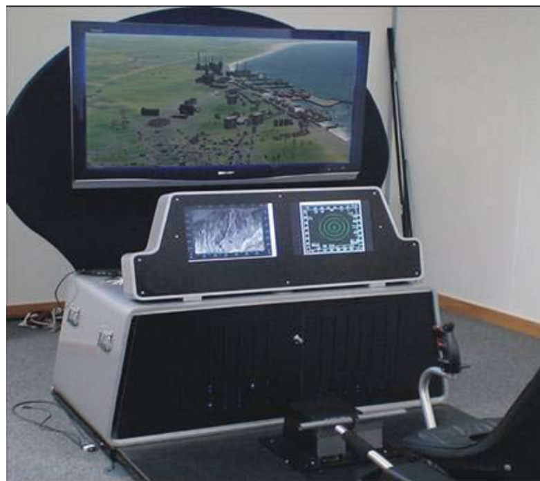
The larger Rotary Wing Simulator consisting of pilot's display, joysticks, foot pedals, and representative collective
